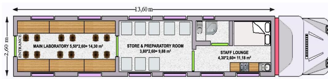
Fig. 6. The plan of the MSL of Mobilim.
